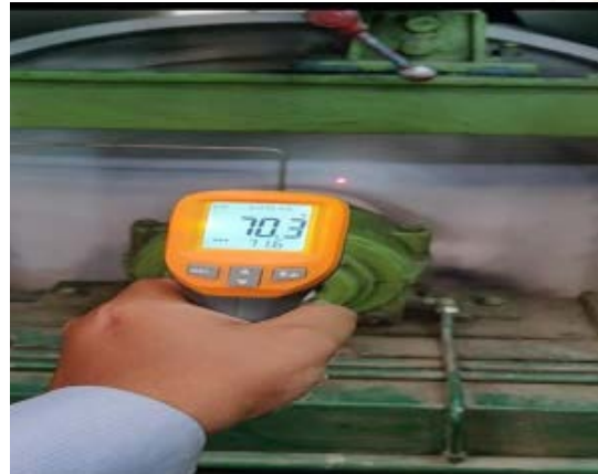
Figure 32 UGAMI HRTI 400 Silver coated temperature 70.3 Deg C
