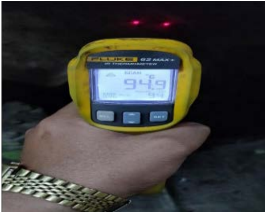
Figure 31 Uncoated Temperature 94.9 Deg C
