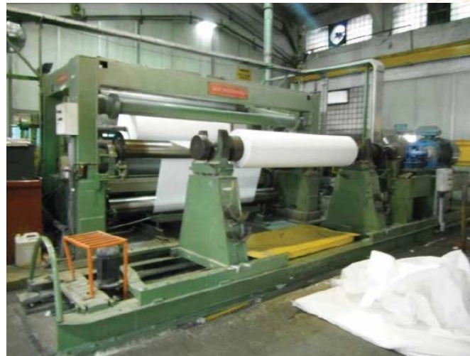
Figure 16 Unwinder with Regenerative Braking motor
