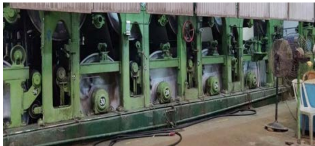
Figure 30 Application of UGAM HRTI 400 Silver on sides of rollers
