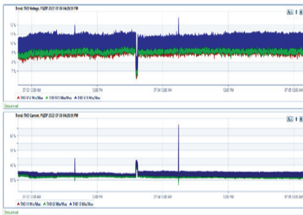
Figure 20 Harmonics on one of the transformers
